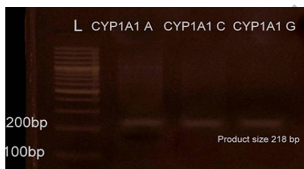
Fig. 5. Gel image showing amplified products for wild type A and allelic variants C, G of CYP1A1.
