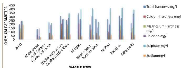
Figure 4: Comparison of chemical parameters in drinking water samples.
