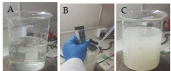
**Figure 1:** Photograph showing the steps of Fabrication of Chitosan nanoparticles A. Dissolving chitosan in deionized water and stirring. B. Adjusting to pH 7 by adding NaOH. C. filtering the formed semi-gel solution.
