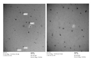
Figure 2: TEM image of spherical Nano-MO with an average size 24.1 nm
