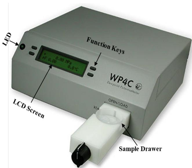
Figure 1: Schematic view of WP4C (Source: Meter Group, 2019).
