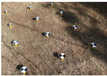
Figure 1: Erosion pipes installation in dense forested area.
