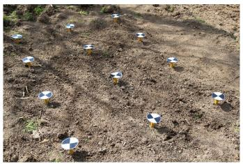
Figure 3: Erosion pipes installation in agricultural land.
