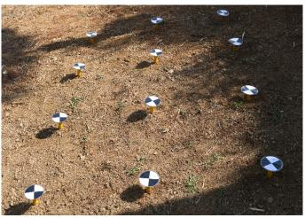
Figure 2: Erosion pipes installation in moderate forested area.
