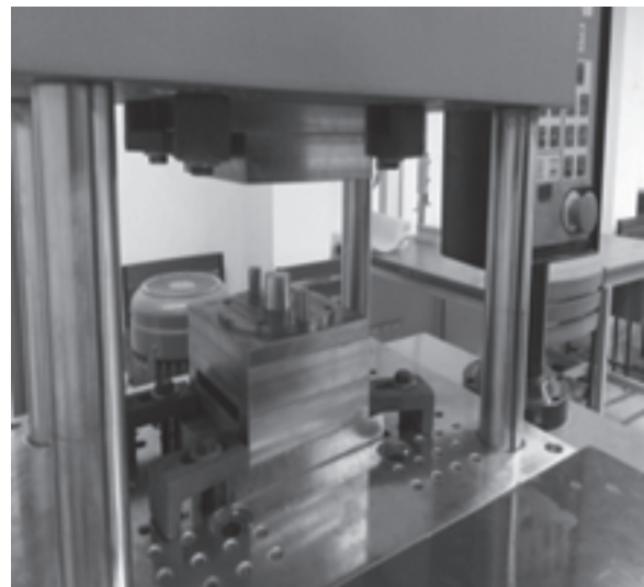
Fig. 19: Ejection of product after solidification
