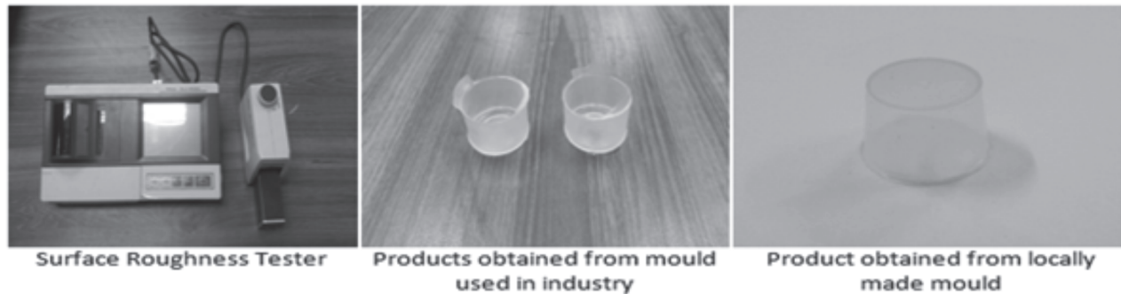
Fig. 20: First picture represent the surface tester, second one is the products fabricated in industry and the third picture is the product fabricated in injection molding machine in our lab
