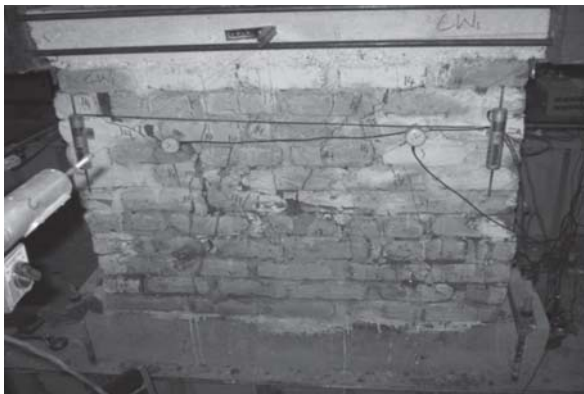
Figure 6: Damage pattern of CW
