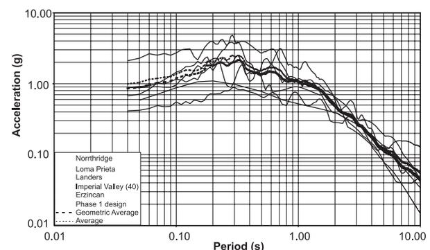
Figure 1: Comparison of acceleration response spectra for scaled earthquake time histories and design response spectra for DLE-horizontal X direction - damping ratio = 5%. Log-log plot
