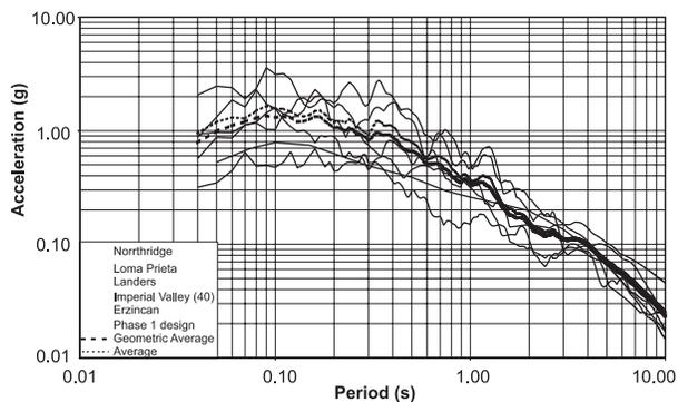
Figure 3: Comparison of acceleration response spectra for scaled earthquake time histories and design response spectra for DLE-Vertical direction - damping ratio = 5%. Log-log plot
