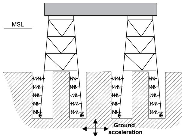
Figure 9: Schematic of soil boundary conditions (T-z springs not shown for clarity)
