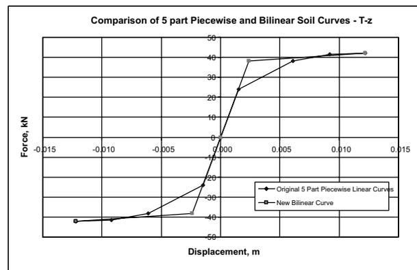
Figure 7: Comparison of 5-part piecewise linear and bilinear T-z soil springs
