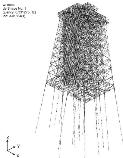
Figure 12: Third mode of vibration (Torsion)
