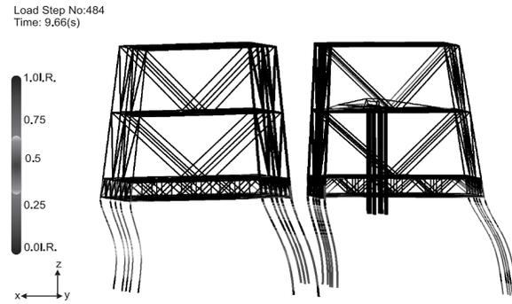
Figure 16: Deformed Shape and Member Utilisations for DLE Landers Event at Maximum Base Shear (Foundation and lower part of both jackets)
