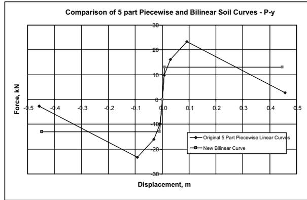
Figure 8: Comparison of 5-part piecewise linear and bilinear P-y soil springs.
