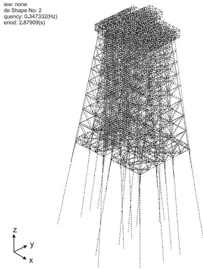
Figure 11: Second mode of vibration (Sway in X direction)
