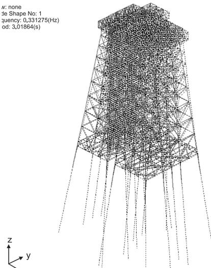
Figure 10: First mode of vibration (Sway in Y direction)
