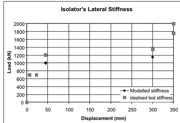
Figure 6: Isolator stiffness used in SAFJAC
