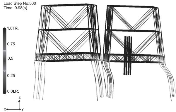
Figure 15: Deformed Shape and Member Utilisations for DLE Imperial Valley Event at Failure (Foundation and lower part of both jackets)
