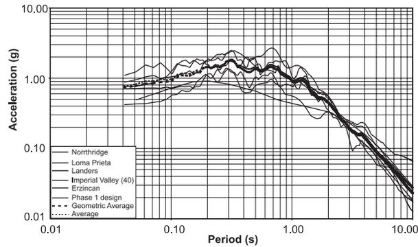
Figure 2: Comparison of acceleration response spectra for scaled earthquake time histories and design response spectra for DLE-horizontal Y direction - damping ratio = 5%. Log-log plot
