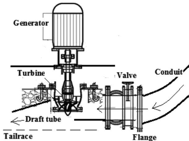
Figure 5: Schematic of the present micro hydroelectric plant
