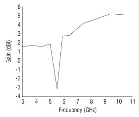
Fig.10 Peak gain versus frequency for proposed MIMO Antenna
