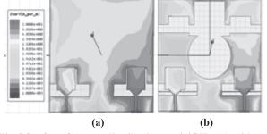
Fig.6 Surface Current distribution at 4.4GHz (a) without spider and pair of lines (b) With spider and pair of lines
