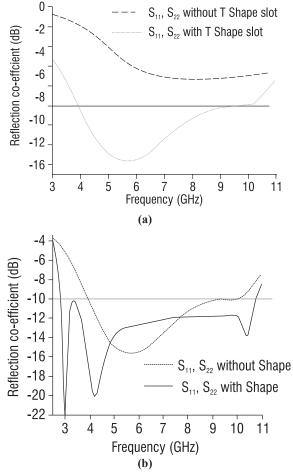
Fig. 4 scattering parameters with and without (a) T shape slot (b) spider shape
