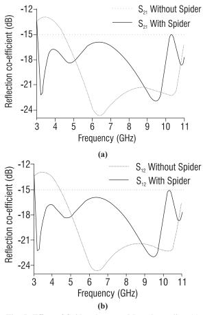
Fig. 5: Effect of Spider shape on Mutual coupling (a) antenna2 (b) antenna1
