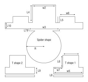
Fig. 2 Back view of MIMO antenna
