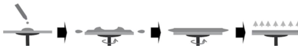
**Fig 1. Spin coating step procedure**
