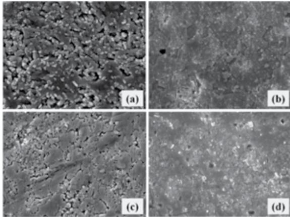
Figure 4: SEM of SAC305 (a) as-casted and thermally aged at (b) 60 °C (c) 100 °C (d) 140 °C
