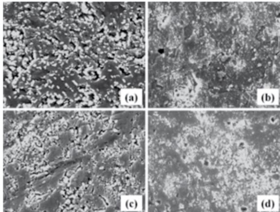
Figure 5: SEM images analyzed in ImageJ (a) as-casted and thermally aged at (b) 60 °C (c) 100 °C (d) 140 °C
