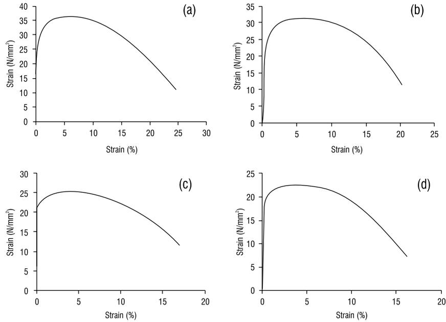
Figure 7: Stress strain curves of SAC305 (a) as-casted and thermally aged at (b) 60 °C (c) 100 °C (d) 140 °C
