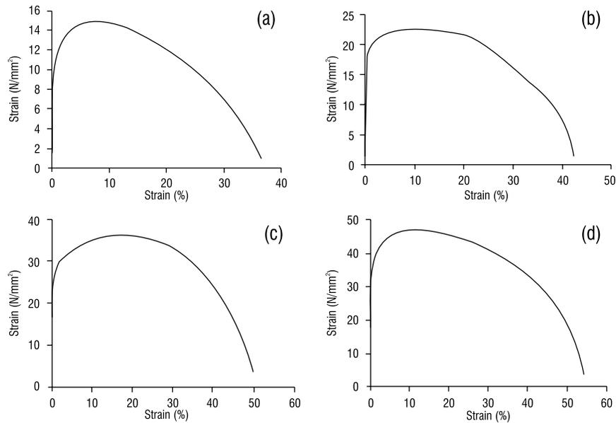
**Figure 8: Stress strain curves of SAC305 under high strain rate (a) 10/s (b) 20/s (c) 30/s (d) 40/s**
