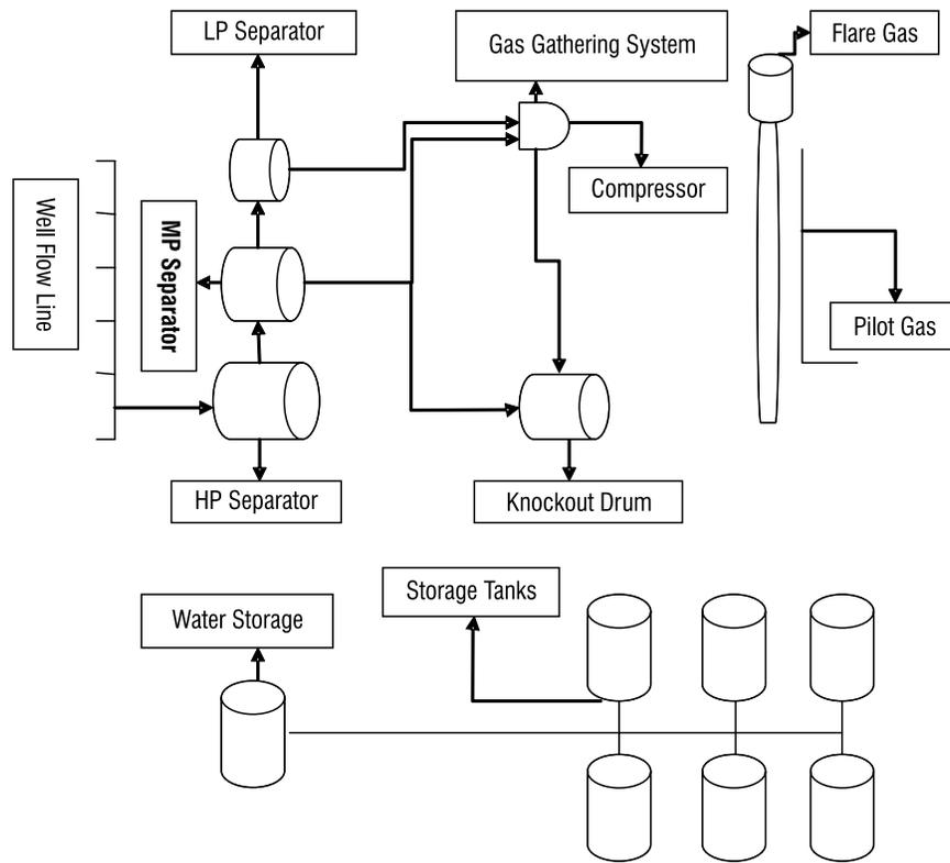
**Figure 1: Plant Gas Flaring Process**
