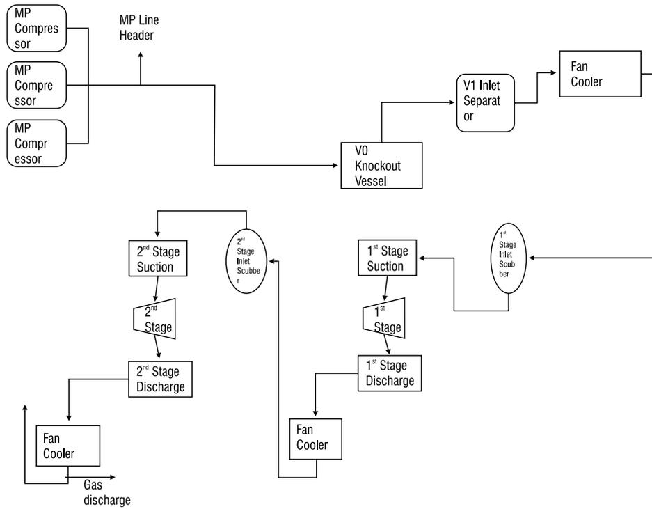
Figure 2: Process flow diagram of the existing system
