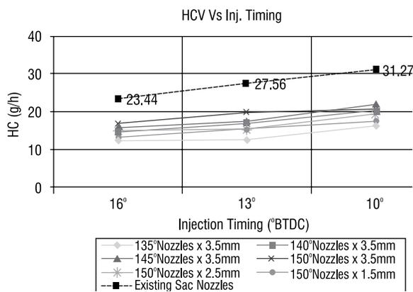
Figure 6: HC emissions at different injection timings
