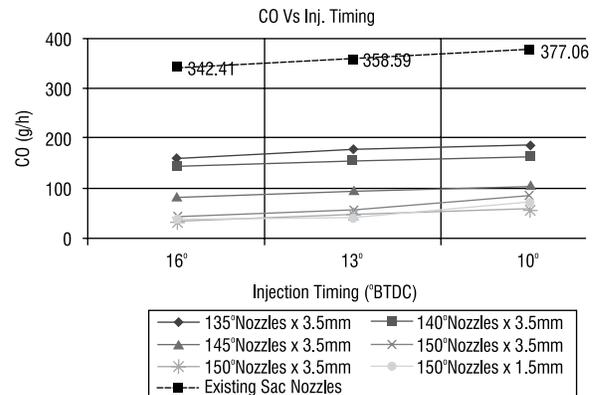
Figure 7: CO emissions at different injection timings
