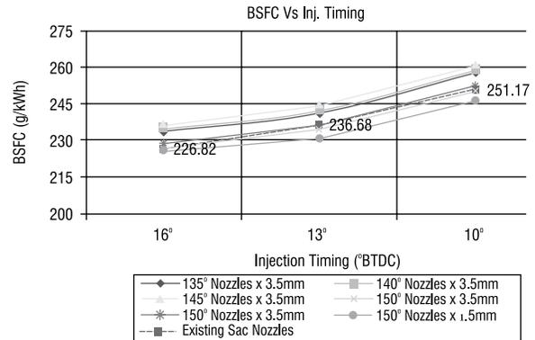
**Figure 2: The variation in BSFC at different Injection Timings**
