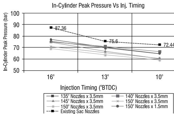
Figure 4: In-cylinder peak pressure at different injection timings
