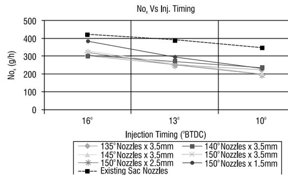
Figure 5: NOx emissions at different injection timings
