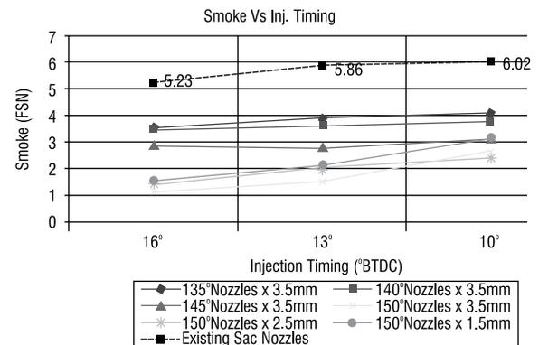
Figure 8: Smoke emissions at different injection timings
