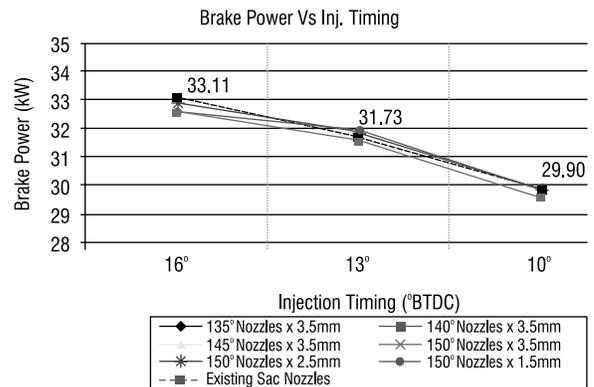
**Figure 3: The variation in Brake Power at different injection timings**
