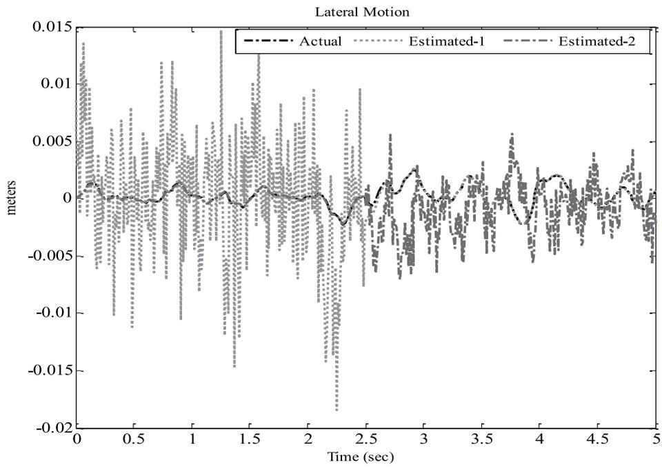
Figure-5 lateral movement for error state estimation of wheelset perturbations
