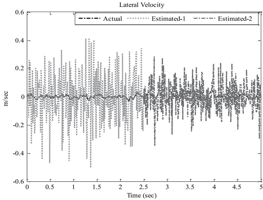
Figure-4 lateral velocity error estimation for wheelset perturbations
