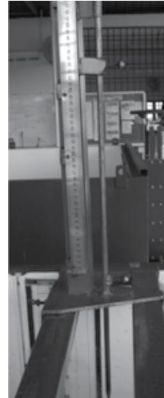
**Figure 4: Vertical Point Gauge**
