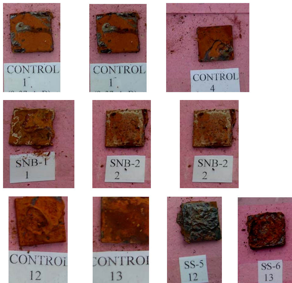
Fig 3. Appearance of the mild steel coupons (2×2cm) exposed to nutrient broth (control) and different cultures for one month period. Excessive corrosion products on the surface of experimental coupon as compared to the respective control ones are evident.
