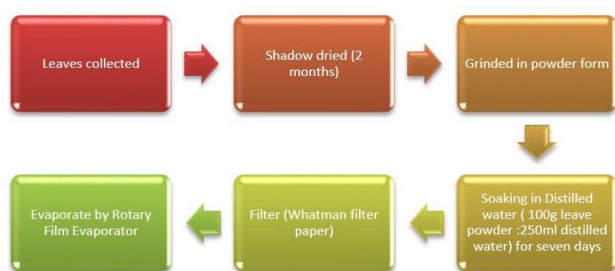
Figure 1: General flow diagram showing solvent extraction.
