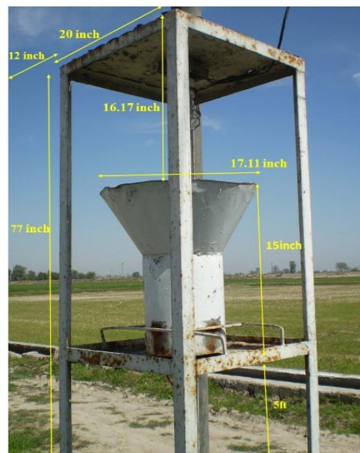
Figure 1: Schematic diagram of the light trap design.
