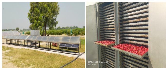
Figure 2: Solar-cum gas fired dryer.
