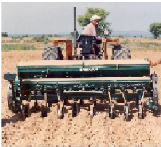
Figure 2. Rapeseed drill with packing wheels
