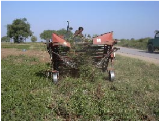
Figure 16. Digger-inverter in field operation
