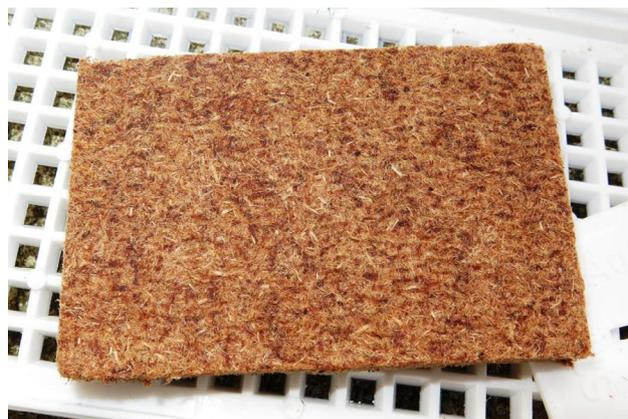
Fig. 2. Fragment (30 g) of the porous strip evaporating strip: Detail of porous structure.
