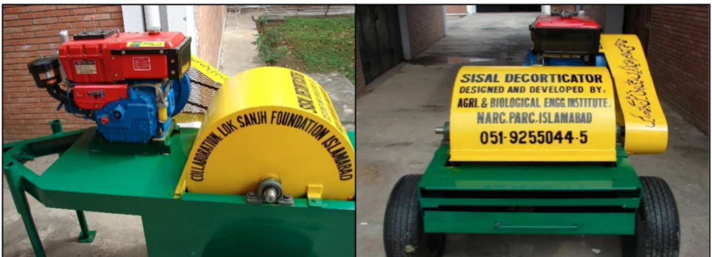
Figure 2: Prototype unit of sisal decorticator.
