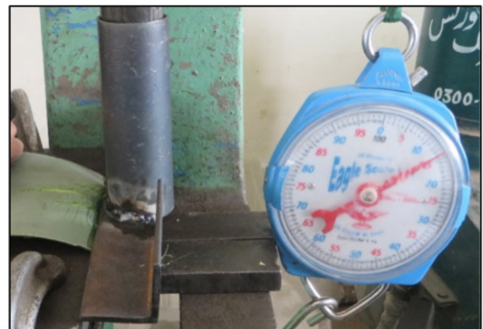
Figure 4: Measurement of sisal decortication resistance.
