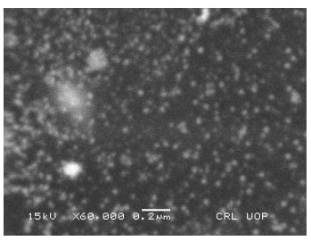
Figure 3: SEM Image of Ag-Lapachol nanoparticles.
