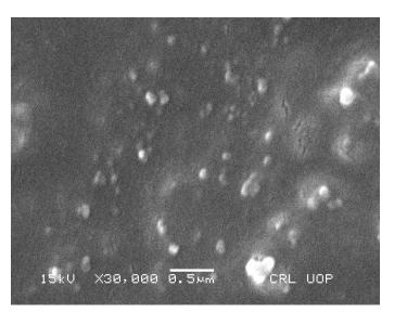
Figure 2: SEM Image of Cu-Lapachol nanoparticles.
