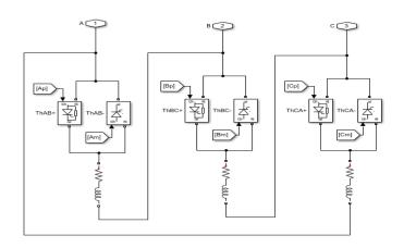
**Figure 1:** three phase thyristor switched capacitors with added line inductance.
