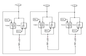
Figure 2: Three phase thyristor controlled reactors.
