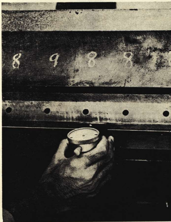
Fig. 9. Setting the horizontal nosebar gap with laboratory designed Setting Gauge.
