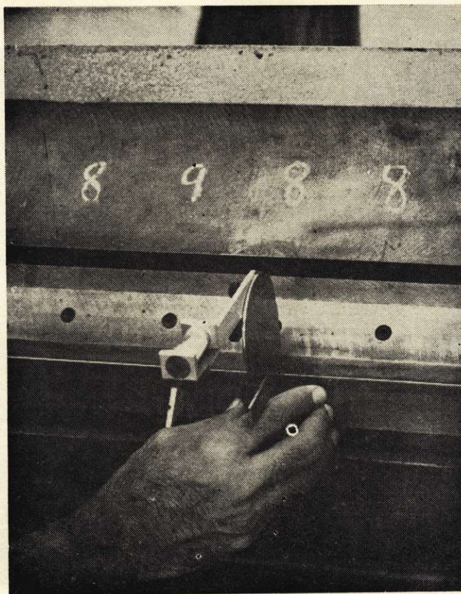
Fig. 7. Adjusting the knife angle with the help of bevel protector.
