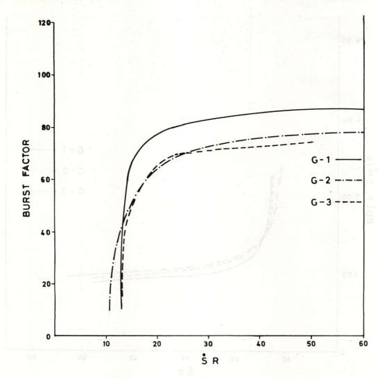
Fig. 2 Comparison of burst factor of handsheets from three groups of trees at different freeness levels
