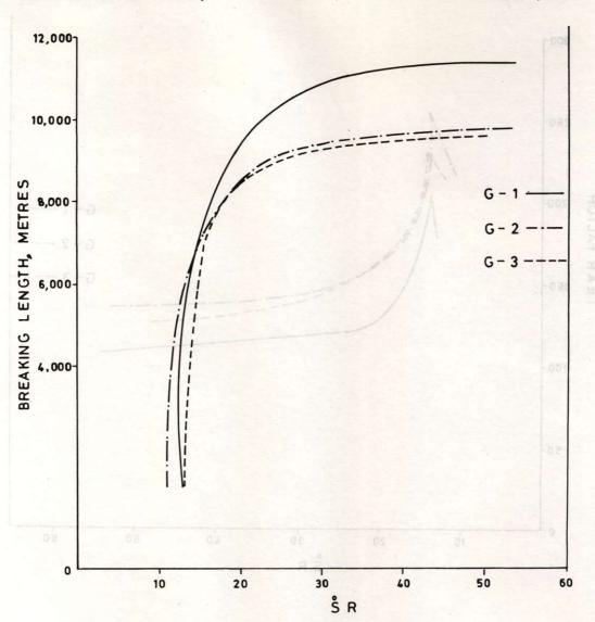
Fig. 3 Comparison of breaking length, m, of handsheets from three groups of tree at different freeness levels
