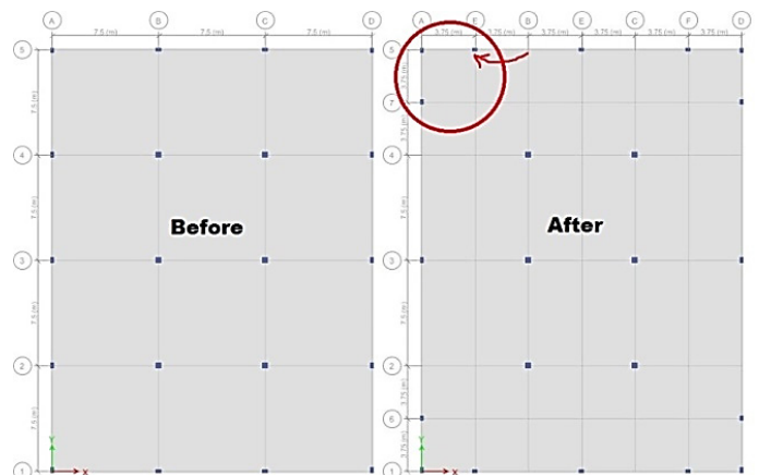
Figure 5: Columns near corner edge brought closer.
