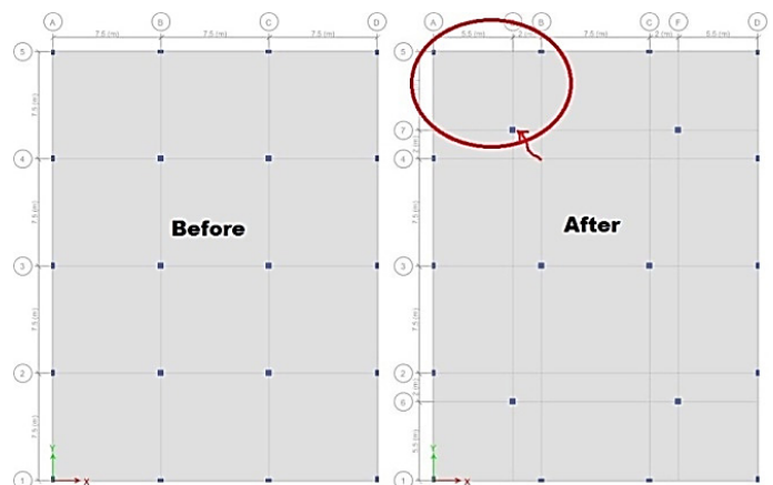
Figure 6: Diagonally located column brought closer to the corner.
