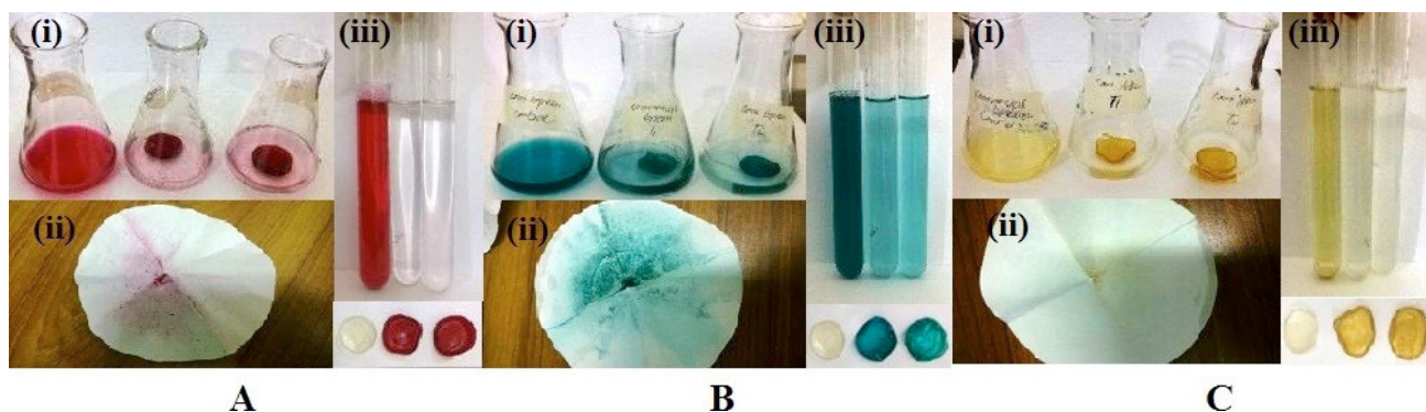
Fig. 5. The figures A, B, C shows the separation of the commercial dyes from the waste water after treatment with chitosan starch based nanocomposites. The flocculation was removed by filtration. In each case dye particles are visible on filter paper (A ii, B ii, C ii). The filtrate in the test tube (A iii, B iii, C iii) clearly shows the removal of dyes from commercial samples. Nano composites before and after treatment are also shown underneath the test tubes.
