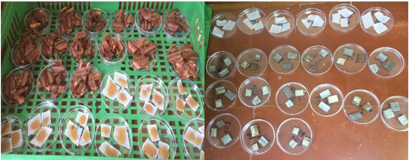
Figure 1: Different coupon surfaces (metal, plastic and cooling pads) used in this study.
