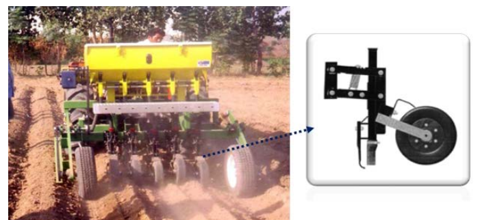
Figure 9: Seeder sowing two rows of wheat on narrow bed with row spacing of 20 cm. Insert shows diagram of the press wheel and seed placement component.
