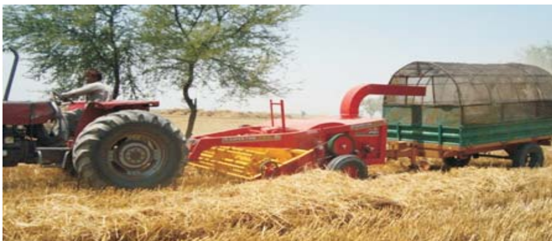
Figure 1. Improved wheat straw chopper in operation in the field at first site
