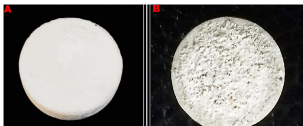
Fig. 5. The surface of the \beta -CPP sample. (A) before immersion in SBF, (B) after two weeks of immersion in SBF.
