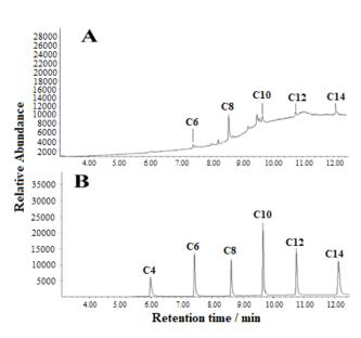
Fig. 2. Sterile culture extracts of marine snow isolated bacterium *C. freundii* B1 (A) and the mixture of six standards (synthetic AHLs) with their retention times (B) at m/z 143 in SIM mode of GC-MS.
