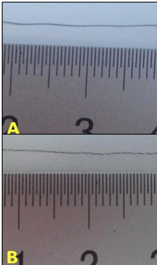
Fig. 1. Wire making. **A**, a diameter of 0.02 mm of ordinary steel wire; **B**, making the wire bent.
