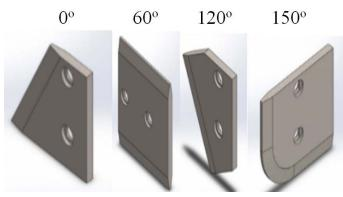
**Figure 1:** Blades with 0°, 60°, 120° and 150° lifting angles used for the comparison.
