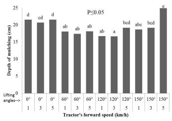
**Figure 6:** *Effect of tractor's forward speed and blade lifting angles on the depth of mulching.*
