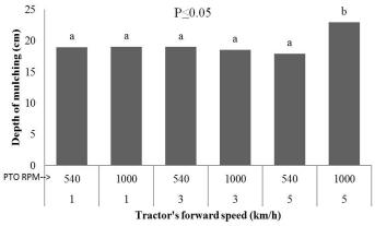
**Figure 8:** Effect of tractor's forward speed and tractor's PTO speed on the depth of mulching.
