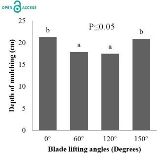
Figure 3: Effect of blade lifting angles on the depth of mulching.
